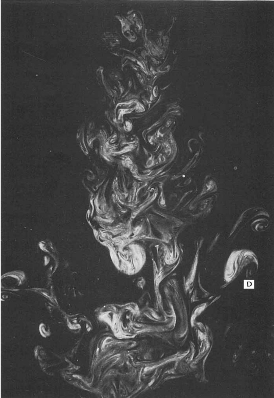
FIGURE 2. A two-dimensional slice of a turbulent jet at a nozzle Reynolds number of about 4000, obtained by the LIF technique. The entire extent of the CCD array ( 1300 \times 1000 pixels) was used to obtain this image. The region imaged extends from 8 to 24 diameters downstream of the nozzle. A Nd:YAG laser beam shaped into a sheet of about 250 \mu\text{m} thickness using a suitable lens was directed into the water tank into which the nozzle fluid containing small amounts of a fluorescing dye was emerging in the form of a jet. The laser had a power density of 2 \times 10^7 \text{ J s}^{-1} per pulse and a pulse duration of about 10 ns.
